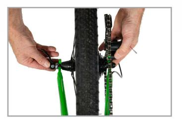
Step 3. Loosen and open the rear wheel quick release clamp. Pushing your derailleur slightly towards the back of the bike, pull up the wheel from the grooves of the frame.
