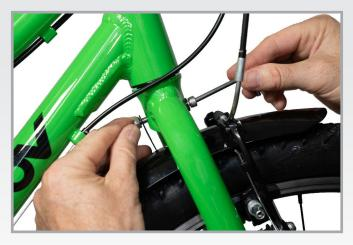
**Step 3.** Slide the screw A x1 into the fork hole from the front to the back of the bike, taking care to position the washer between the allen bit and the paint. Secure the mudguard in the lowest position by tightening the self-locking nut at the black mounting bracket.
