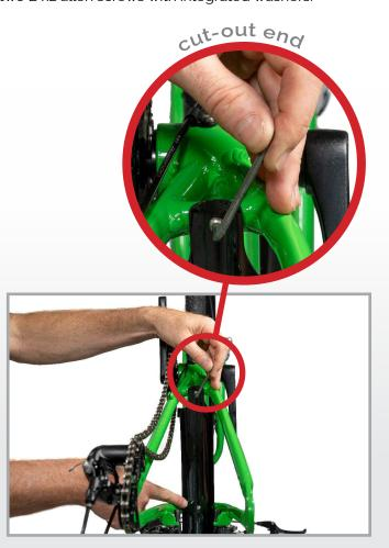
Step 5. Secure and tighten, using two C x4 screws, the black bracket at the screw threads at the rear end of the frame.
