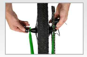
By gradually releasing the derailleur, fit the axle of the wheel at the grooves of the rear legs of the frame.
