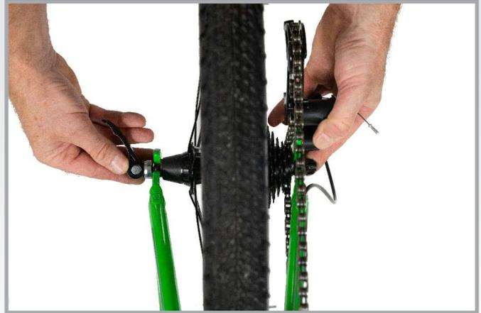
By gradually releasing the derailleur, fit the axle of the wheel at the grooves of the rear legs of the frame.
