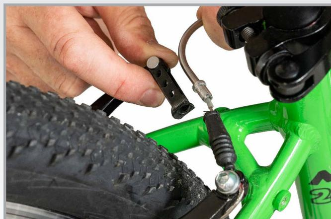
**Step 2.** Unscrew the rear brake cable at the aluminum elbow tube to release both rear brake arms.
